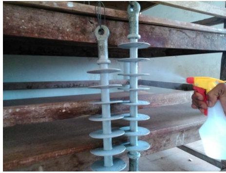
Fig.3 Artificial Salt Contamination by spaying method
